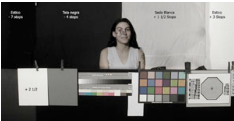
In this image you can see the values of light reflected from the value Normal (medium grey 18%). 24fps/ 172,8° / T 5.6
